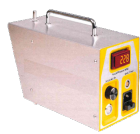
Salt particulate generator
